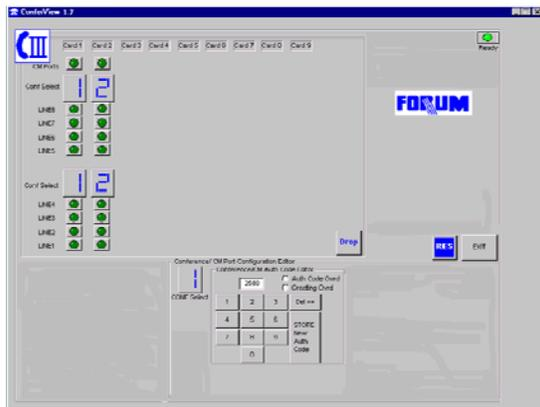
The ConferView Console includes GUI Interface for control/monitoring via PC console (user provided) OR, remotely via modem. This new option can be used alone or to enhance Confer III Remote Administrative functions:
